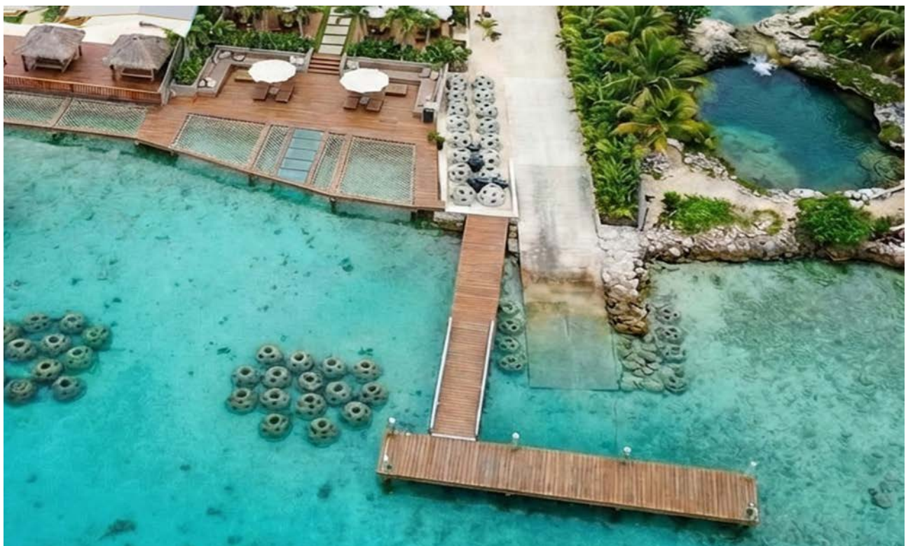
Image 17 | Reefball Deployments can be placed anywhere to help improve habitat complexity including under jetties, beside seawalls to offset any damage created from the construction.
